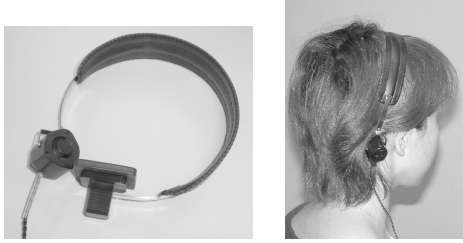
Figure 3: The ceramic vibrator of the BCUHA attached to the mastoid with a hair band-like device
