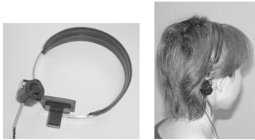
Figure 1: Ceramic vibrator of the BCUHA attached to the mastoid with a hair band-like device
